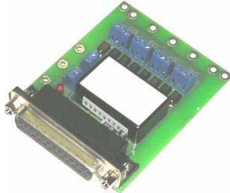
Figure 1. 25-Pin D-Sub Connector Kit with Strain Relief
